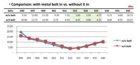
•INCH SQ HT reads SAME, regardless of whether fastened with metal bolt in a hole (located at center of tags) or not, because it was originally designed as assuming metal bolt in. Stainless steel M4 bolt with round head is best fit for INCH SQ HT.
